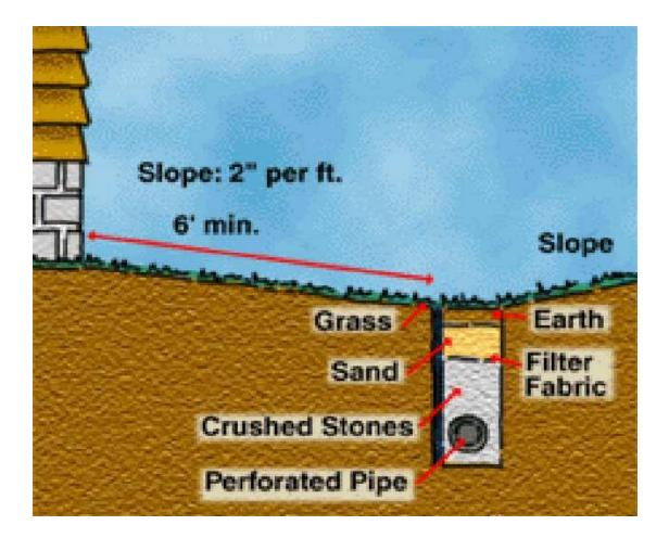
The Drainage trench and swale is created between two slopes to redirect ground surface and subsurface water flows and thereby reduces moisture at the immediate soils around the foundation.
