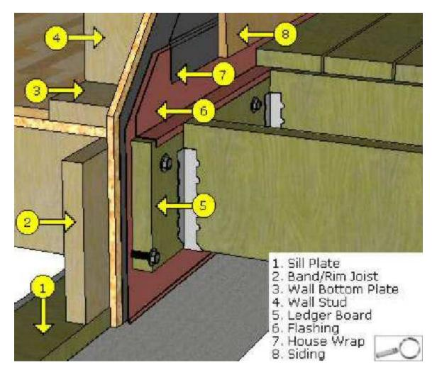
In this photo, note how the House Wrap (item #7) overlaps the flat wall flashing and a second flashing called the Ledger Board (item #5) Cap Flashing (item #6). This method will prevent moisture damage at your house wall sheathing and floor framing areas, however you will rarely ever see a contractor install the Ledger Board Cap Flashing.
